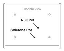
while wearing a broadcast headset, or separate headphones and microphones. Ideally, this adjustment is made with two people on headsets, after setting mic and headphone levels for broadcast. To adjust intentional sidetone level, insert a small flat blade screwdriver into the Sidetone level trim pot and adjust to desired level. Replace the hold plug when finished.
