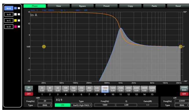
VariQ high pass in freq 1kHz, Q 3.0 (yellow curve: phase)
