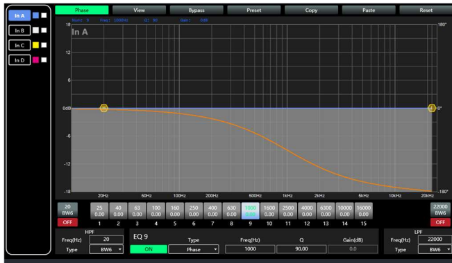
Phase filter in freq 1kHz, Q 90 degree (yellow curve: phase)
