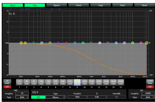
Allpass-1 in freq 1kHz (yellow curve: phase, 90 degree) Application: different speaker
