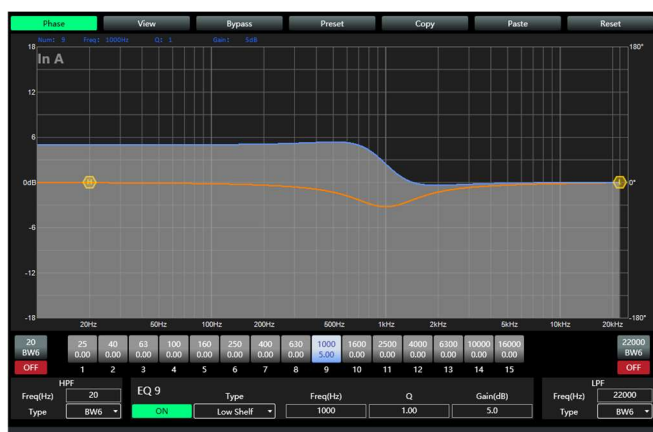
Low shelf in freq 1kHz, Q 1.00 Gain 5dB (yellow curve: phase) Application: musical instruments
