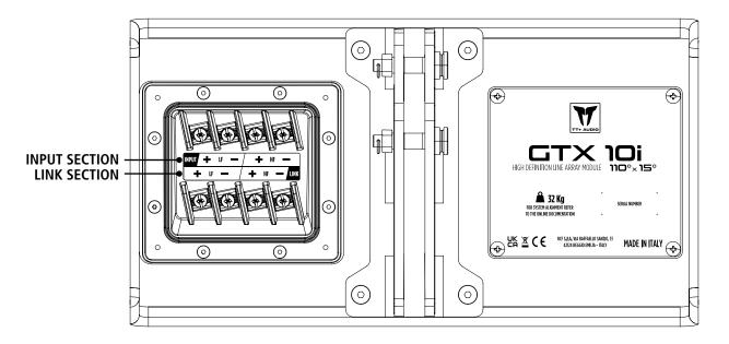
The upper section of the connection board base receives the signal; the left carrier are for the Low Frequencies and the right carriers are for the High Frequencies.
