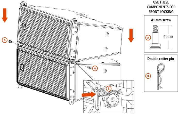
Insert a cotter pin over both screws.
