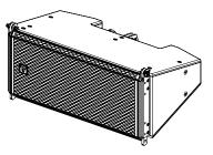
GTX 10Wi 2 x 10" Neo Woofer 4.0" Neo Compression Driver Coverage angle: 110° H x 30° V 32.5 kg / 71.65 lbs
