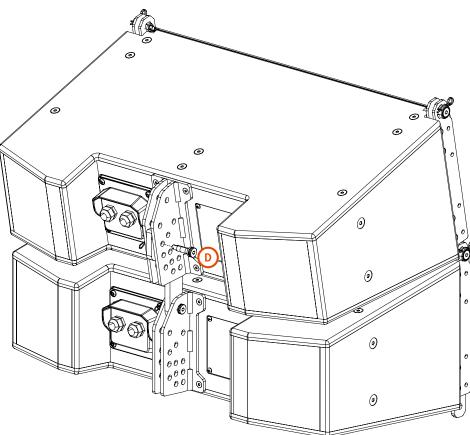
On the other side secure the screw with its nut. Once the screw has been tightened, insert a single cotter pin (E) on the screw as shown in the picture.
