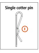
Once the screw has been tightened on its nut, insert a single cotter pin  $(\mathbf{E})$  on the screw as shown in the picture.
