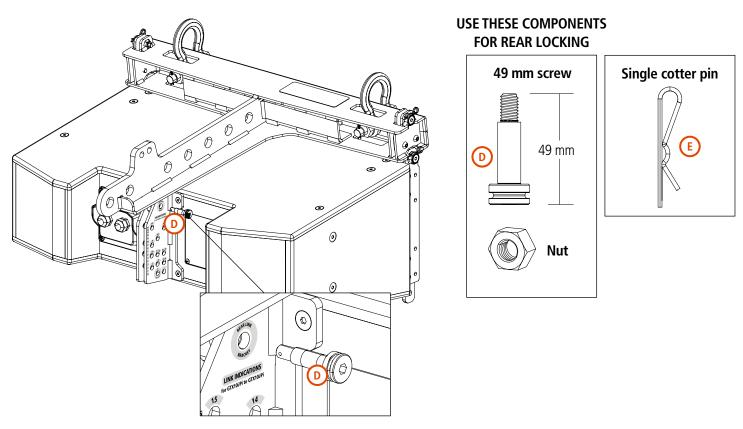
Once the screw has been tightened to its nut, insert a single cotter pin as shown in the picture
