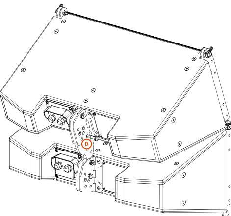
On the other side secure the screw with its nut. Once the screw has been tightened, insert a single cotter pin (E) on the screw as shown in the picture.
