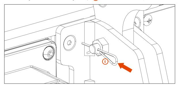
IMPORTANT NOTE: All screws and nuts used to connect modules and flybars must be blocked with a threadlocker like LOCTITE 243 (or another product with similar characteristics).
