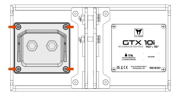
The left rear panel is covered by a plastic contact protection cover. Remove the four screws to remove the plastic cover and to expose the connection board base.
