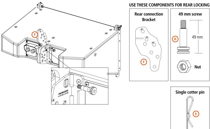
Once the screw has been tightened on its nut, insert a single cotter pin (E) on the screw as shown in the picture.
